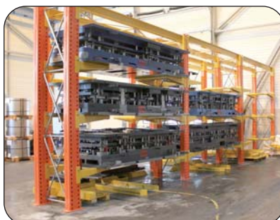
MAXI-CANTIBLOC®, total capacity: 37.5 tonnes (12.5 tonnes per tool)
