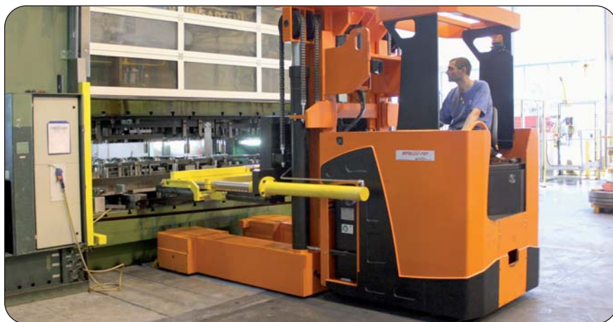
Tool loaded onto 1,000-tonne mechanical press
