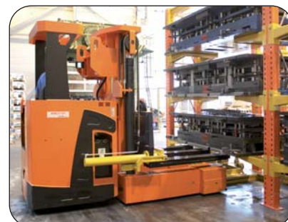
Tool taken up and stacked, without manual intervention
