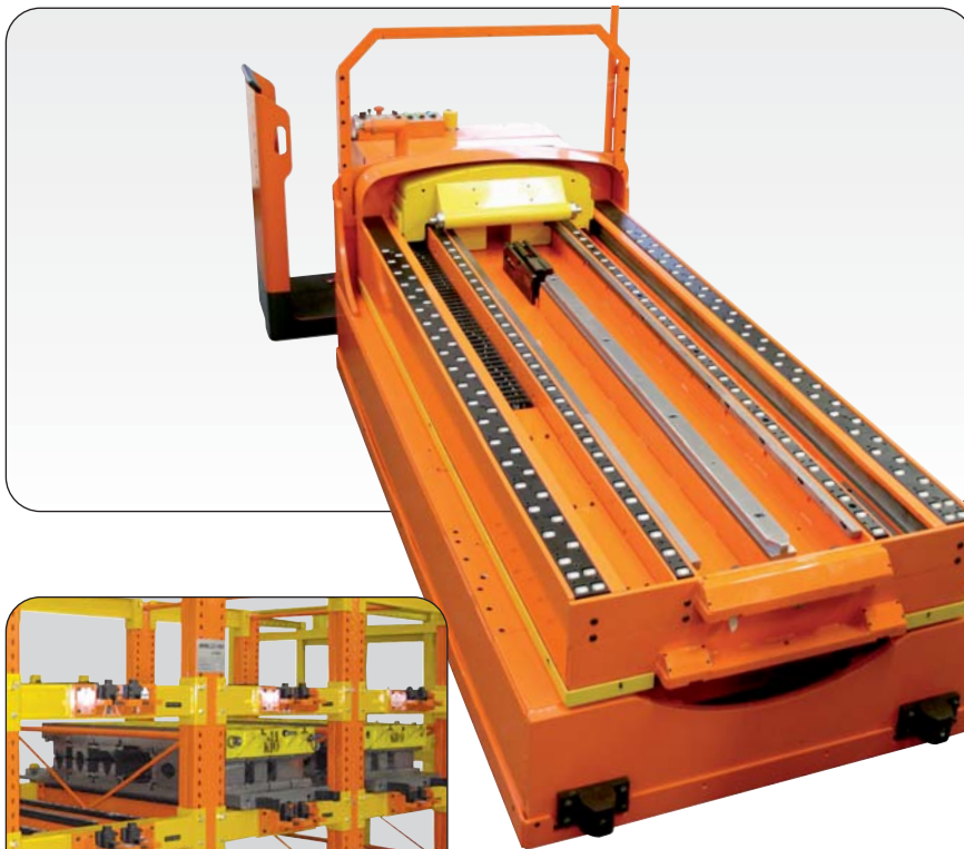
Plate for 2 tools with retractable rollers
