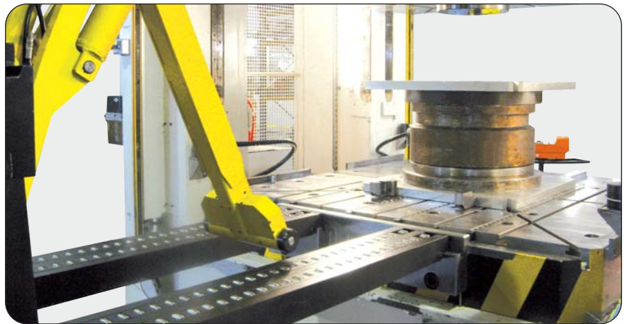
Tool loaded onto 1 000-tonne hydraulic press, fitted with Rotobloc-PSP TRANSROLLER® rolling elements inside press table
